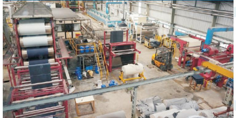
Fabric Processing: We have State of the art Processing Machine. i.e. Kuster Singing, Kuster Desizing, Pad Steams with over Dyeing Facility, Kuster Mercerizing Machine. We have wet finishing machine with washing facility.
