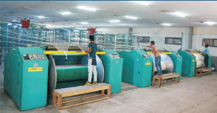
We Have world class warping facilities in separate room with fully computer control and PLC base high speed machine with photo optical stop motions, safety guards, fluff protector, fluff suction and traveler cleaner.
