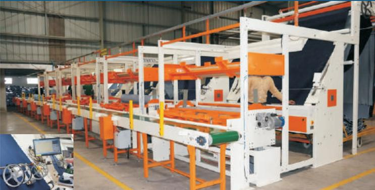
Inspection and packing machines are latest and accurate machines for fabric checking and packing with accurate length measuring device, weighing scale, auto doffer, fabric roll conveying system, damage recording software with display.
