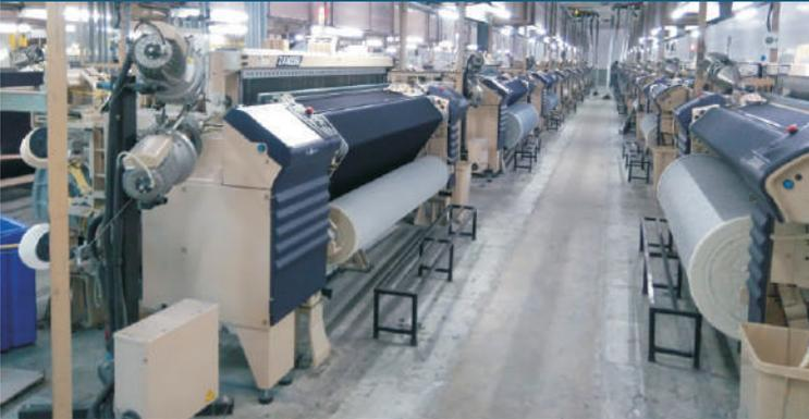
We have Latest Version Picanol (96 Nos.) Tsudakoma (96 Nos.) Air jet Machine with cam and Dobby Shedding motion. We produce various type of weave Combination. i.e. 2/1, 3/1 knitted and Dobby weave denim fabric.
